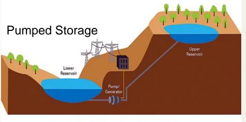
Excess electricity is used to create gravitational potential energy
